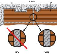
When laying 2 panels side by side in the direction of their length, make sure you start from the same side so that the joints of the panels are in line.
